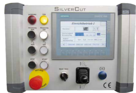
Control panel with touch Display and joysticks for all servo axes of the cutting wheel.
