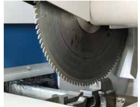
The robot removes a single blank and, following type-specific processes [e.g. deburring, turning], inserts it into the saw.
