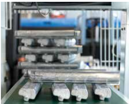
The turntable is manually stocked with blanks by the plant operator.
