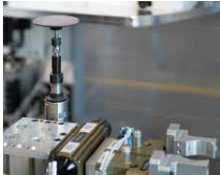
The robot removes a single blank and, following type-specific processes [e.g. deburring, turning], inserts it into the saw.
