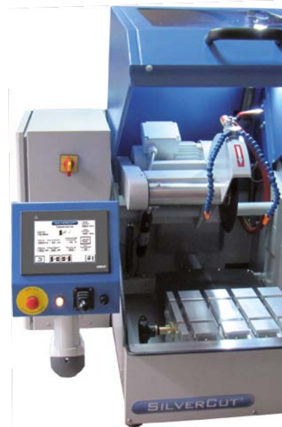
Fig. 1: Password-protected set-up menu for travel paths, maximum speed and end positions
